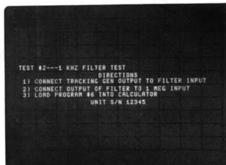
HP 3585A displays detailed instructions for an automatic filter test downloaded from an external computer.
